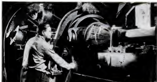
ARMORING MACHINE spins protective sheath around cable first built in 2,300-foot sections. Later these were spliced together and fed into machine.
